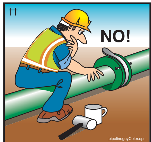
Figure 93 Never straddle or sit on a pressurized pipeline
