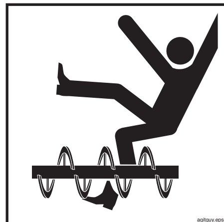
Figure 81 Lifting hopper grate exposes the agitator and the concrete valve
