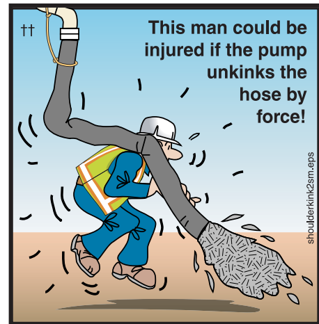
Figure 54 Kinking the hose creates a hazard
