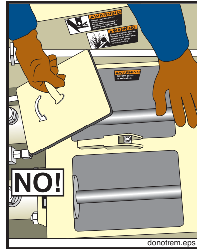
Figure 82 Do not remove the water box covers when the machine is stroking
