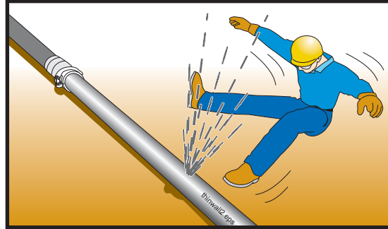
Figure 36 Delivery system components must be able to withstand maximum pump pressure
