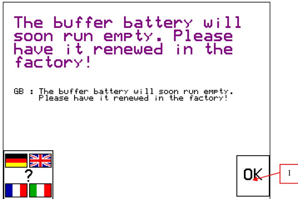
Fig. 2-21 Buffer battery warning
