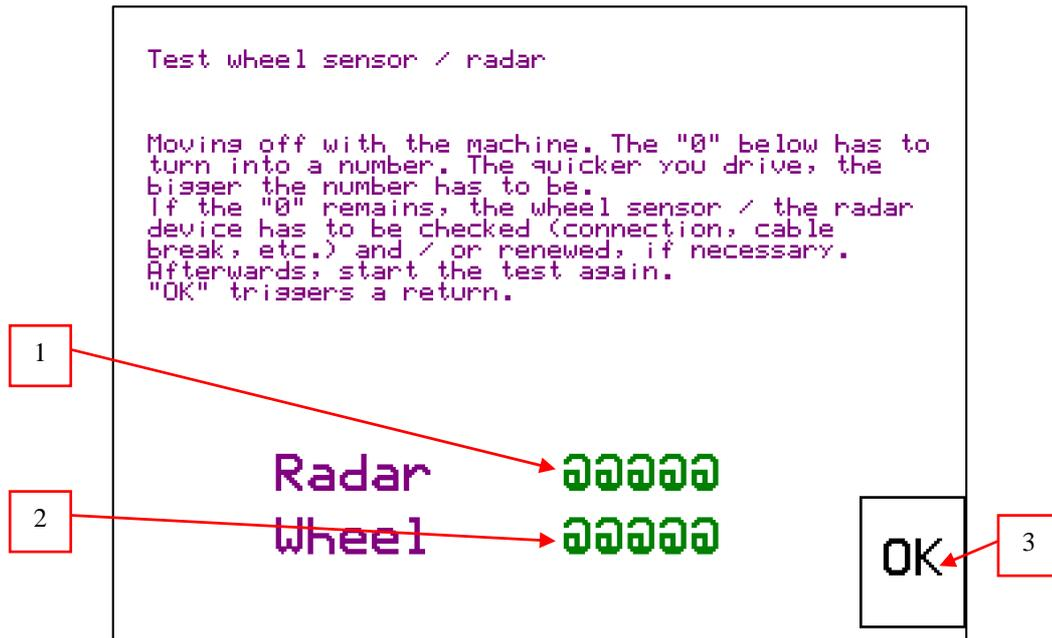
Fig. 2-16 test wheel sensor / radar
