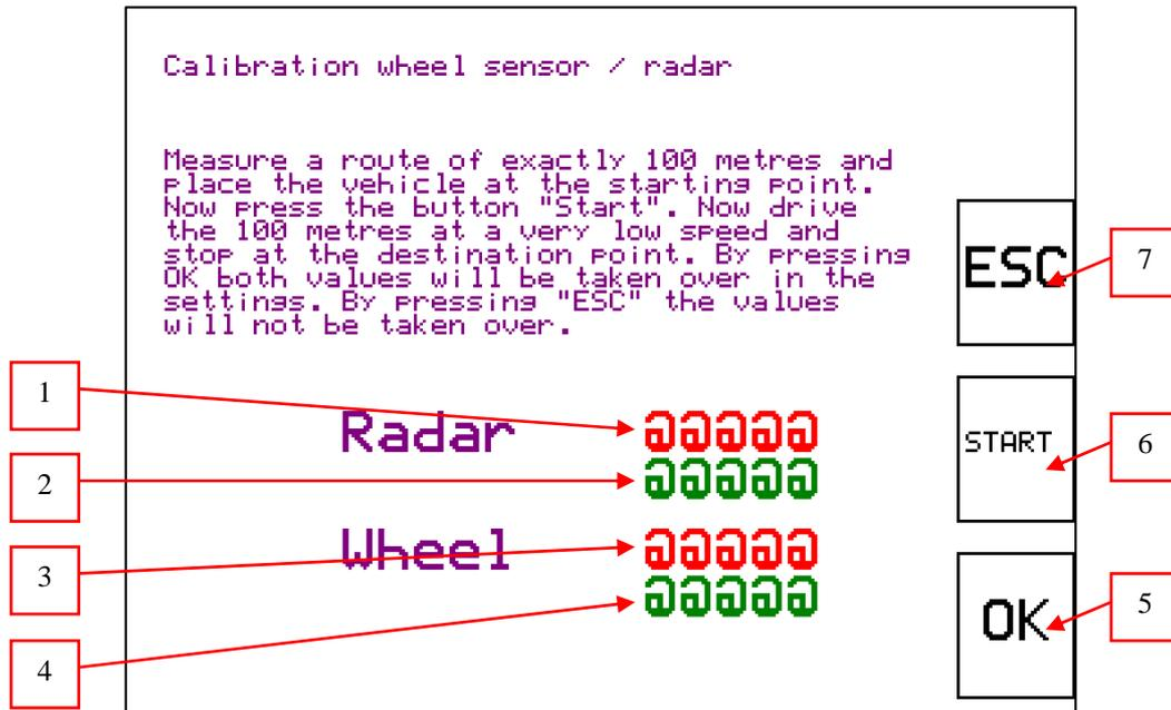
Fig. 2-20 calibration wheel sensor / radar
