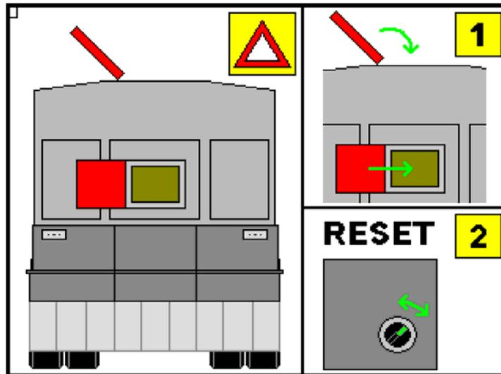
Fig. 2-22 safety switch warning
