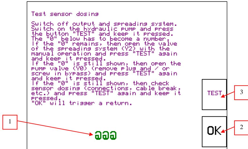
Fig. 2-15 test sensor dosing
