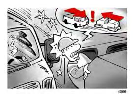
Always select the operator's stand that does not face the traffic flow on the road or that on the construction site.
