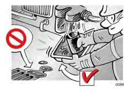
When changing oil or oil filter, collect all waste oil/brake fluid in a suitable vessel!
