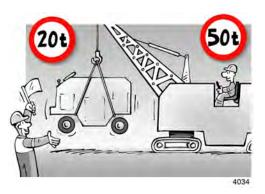
Ensure that lifting devices are strong enough before lifting the machine or any of its components.
