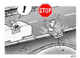
Always be aware of the load capacity of any bridge, cellar roof, arched structure or similar construction before moving the machine
