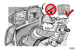
If your machine is equipped with a camera / monitor system, adjust the monitor correctly for easy and glare-free viewing.
