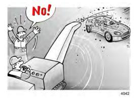
Always select a suitable conveyor speed so that the spreading substance is ejected under control.
