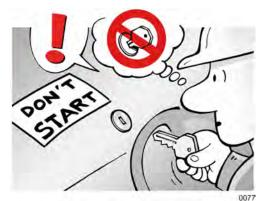
Affix a warning sign on the operator's station prior to starting service and maintenance work to prevent unintended start-up. Remove the ignition key.
