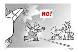
Always ensure that no-one is within the danger zone prior to starting-up and while operating the machine!
