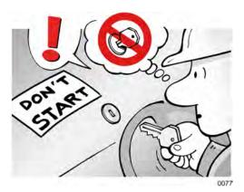
Never start the engine or operate the controls if there is a warning sign attached stating that they are not to be operated! Start and operate the machine from the operator's station only.
