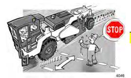
Become familiar with the machine's stopping distance, and always select a safe speed for operation and transport!
