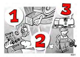
Always stop the engine prior to leaving the operator's station and always secure the machine against rolling away or unauthorized operation!
