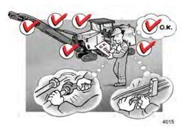
Before starting each shift, walk around the machine and inspect for leaks, loose or missing parts, damaged parts, or parts out of adjustment.
