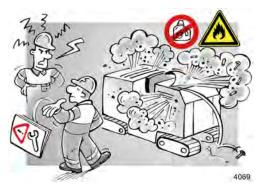
When ether cold start fluid is required, always read the instructions before using. Ether is highly flammable. Do not use ether if the engine is equipped with a glow plug type preheater.
