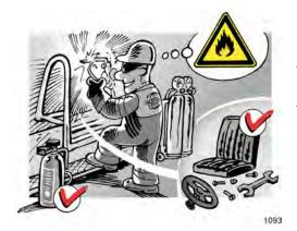
Remove all flammable components near the welding area. After welding, observe the welding area until all components have completely cooled down.
