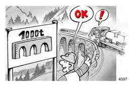
Always be aware of the load capacity of any bridge, cellar roof, arched structure, parking floor or similar construction before moving the machine.
