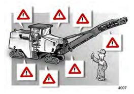
There are areas around the machine which are hard or impossible for the operator to see.
