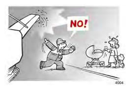
Always ensure that no-one is within the danger zone prior to starting-up and while operating the machine!
