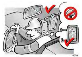
Adjust rear view mirrors so that you can maneuver the machine properly.
