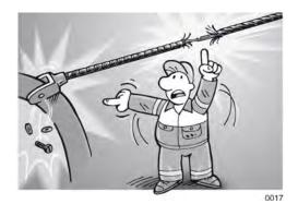
Check that all safety ropes, bolts, spring-clips and other safety elements are correctly installed and in good condition.
