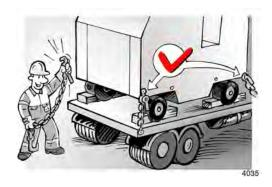
Properly lash the machine to the transportation vehicle!
