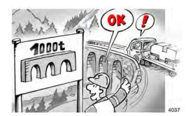
Always be aware of the load capacity of any bridge, cellar roof, arched structure or similar construction before moving the machine.
