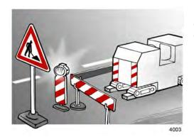
If the machine could interface with the normal flow of traffic, ensure that it is clearly cordoned-off (e.g. warning signs, lights, etc.).
