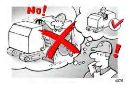
Start and operate the machine from the operator's station only. Prior to starting-up the machine, ensure that no people or obstacles are next to, in front of, behind, under or in the machine.
