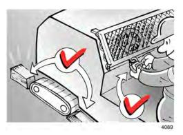
Secure the machine against rolling away and unauthorized operation.
