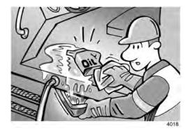
Make sure operator's area, steps and grab rails are clean. Oil, grease, snow, ice or mud in these areas can cause you to slip and fall.
