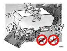
Ensure that the ramps are free of dirt, oil, snow, etc.!
