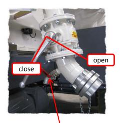
Open the vent valve before removing the filling hose!
