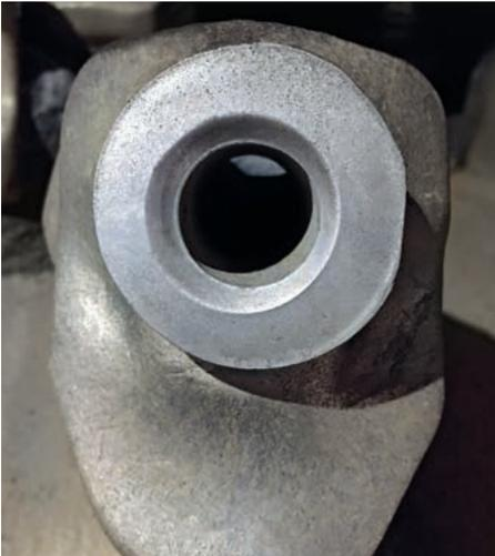
> HT22 quick-change toolholder system after a service period of at least 50 operating hours with a W6/20X pick.
