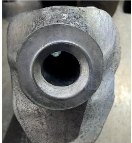
> HT22 quick-change toolholder system after a service period of at least 50 operating hours with a W6/20X<sup>2</sup> pick.
