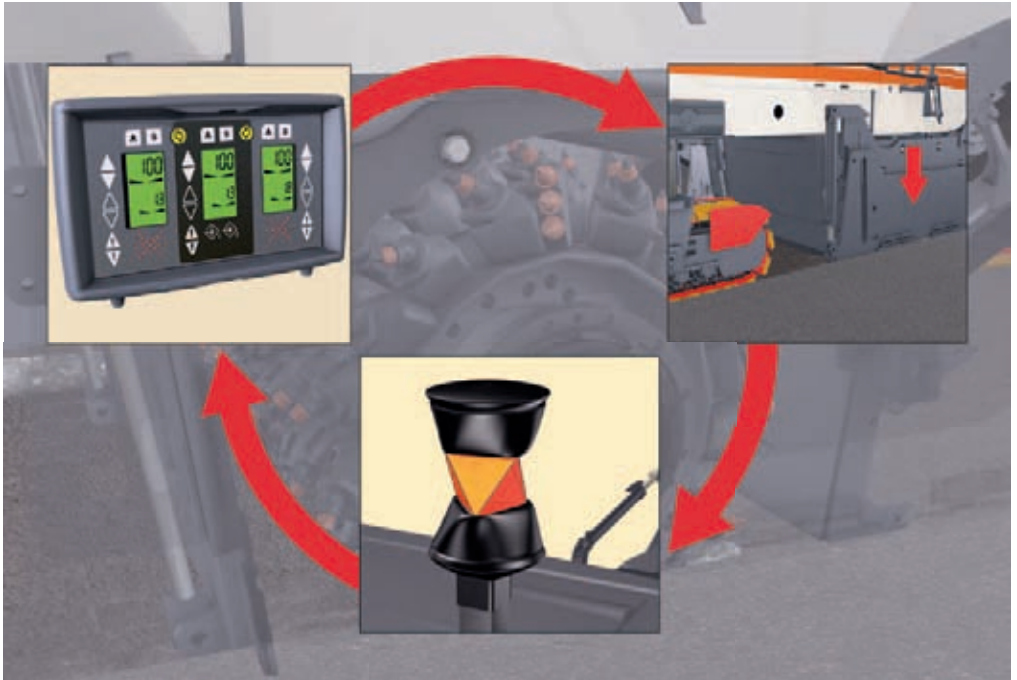
Automated milling depth determination with relative references and corresponding regulation via the levelling control
