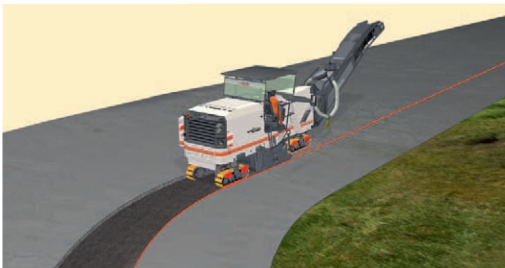
Typical reference line on the surface (red line) when scanning via the side plate.
