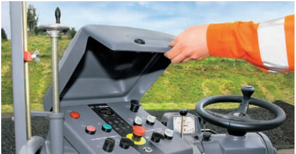
Typical manual machine control on small milling machines
