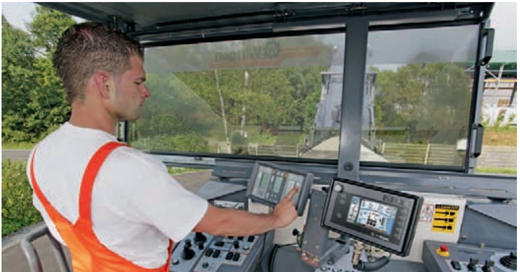
Modern operating and information displays on large milling machines
