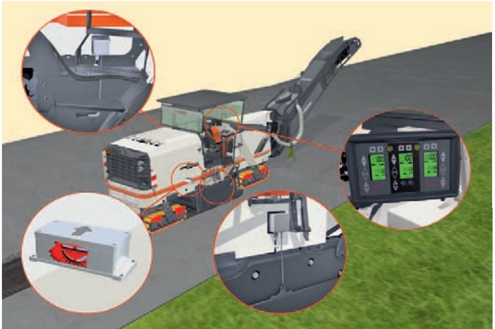
Typical components of a levelling control on large milling machines (cable sensors on both sides, levelling control display, cross slope sensor)
