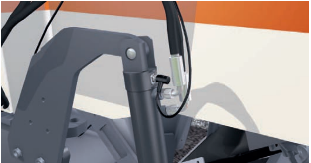
Path sensors in the hydraulic cylinder determine the difference (milling depth) between the side plate and machine chassis.
