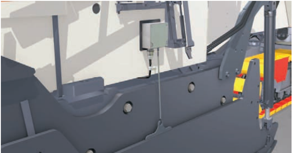
A mechanical cable sensor connected to the side plate with a wire determines the difference (milling depth) between the side plate and machine chassis.
