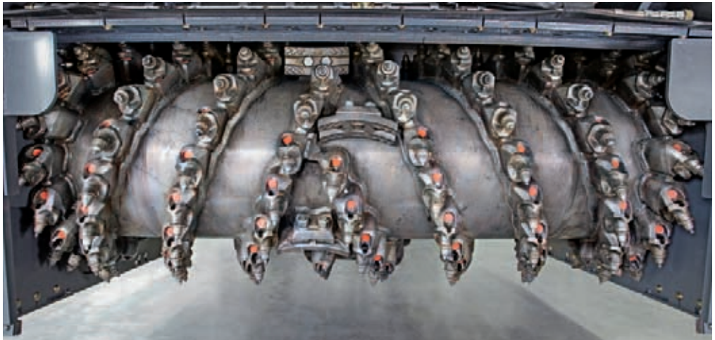
Modern milling drum with exchangeable wearing components
