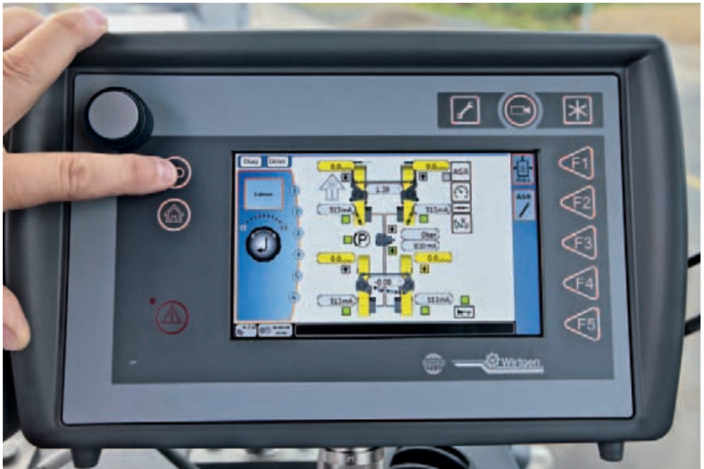
Operating display for travel drive diagnosis on modern large milling machines
