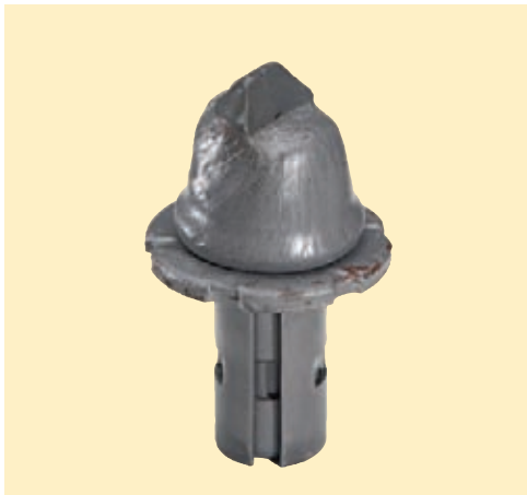
Carbide breakage due to mechanical overload
