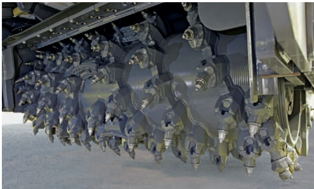
Modern quick-change toolholder system HT22 with considerably greater wear volume
