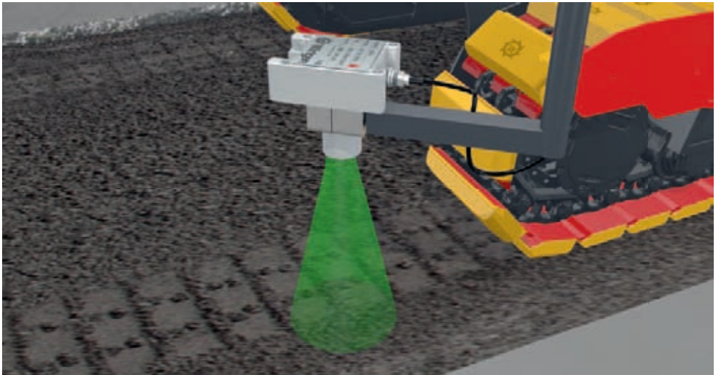
The non-contact ultrasonic sensor determines the distance of the machine to the reference surface.
