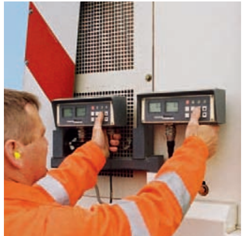
A DLS1 milling depth controller is the operating and control unit for a sensor.
