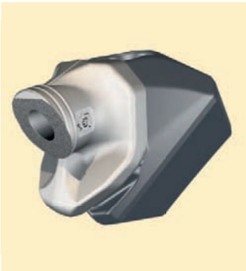
Unfavourable contact surface wear toward the milling drum centre
