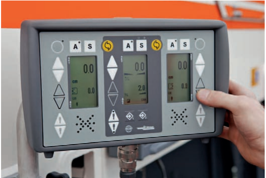
The LEVEL PRO operating display can display three sensors at the same time. The control unit is attached separately at a protected location on the machine.
