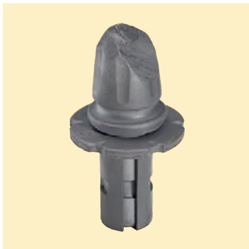
Wear due to insufficient pick rotation
