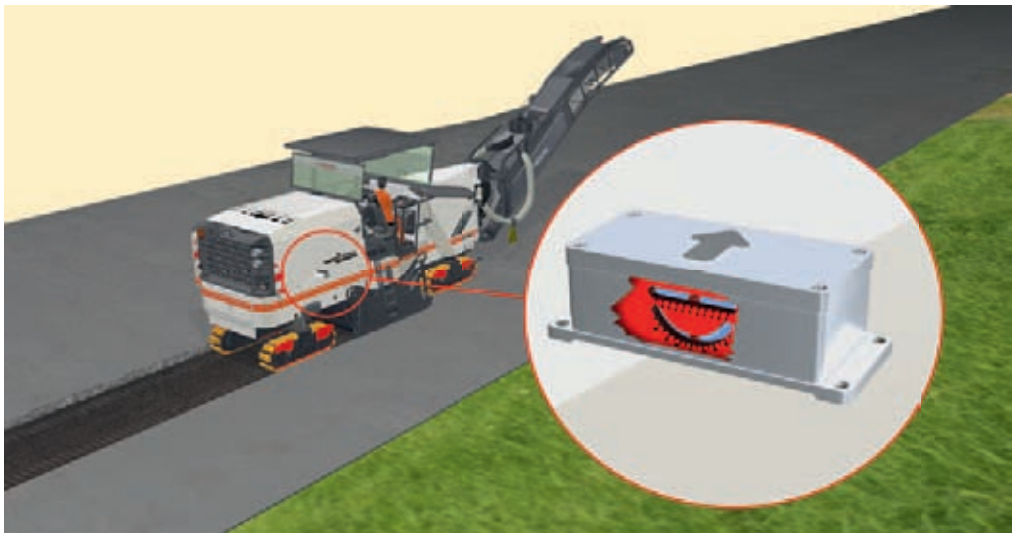
Absolute gravitation reference for determining the cross slope
