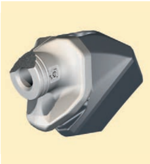
Worn toolholder due to pick loss
