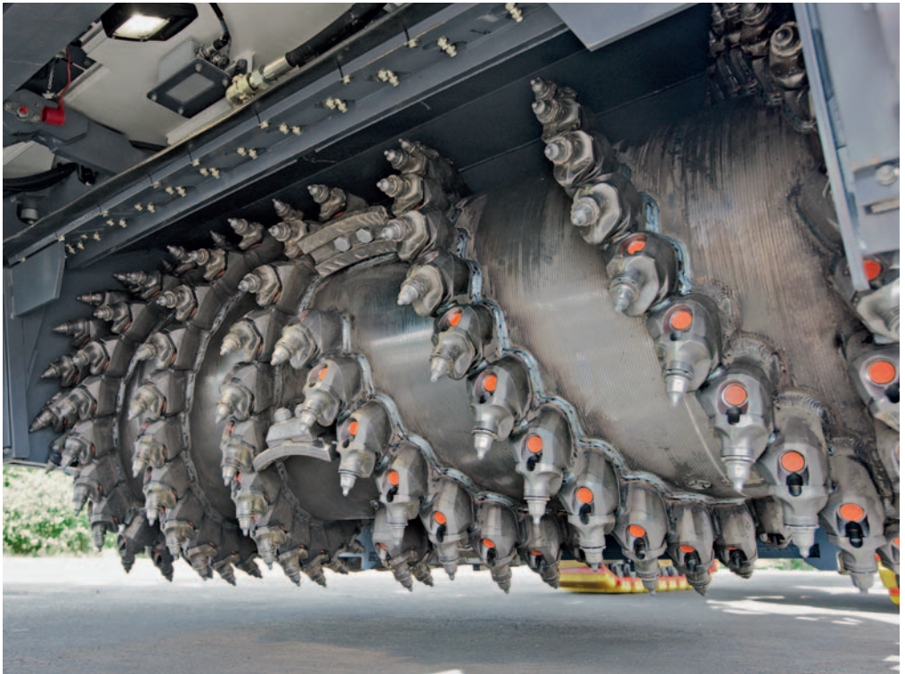
Standard milling drum of a large milling machine with exchangeable toolholders
