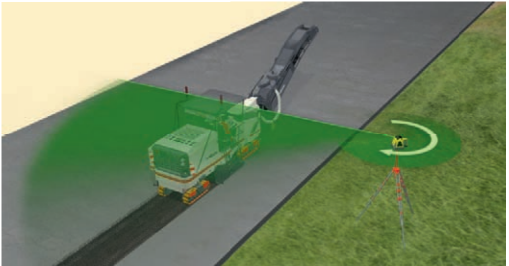
Laser reference level (green) for implementing a level milling depth
