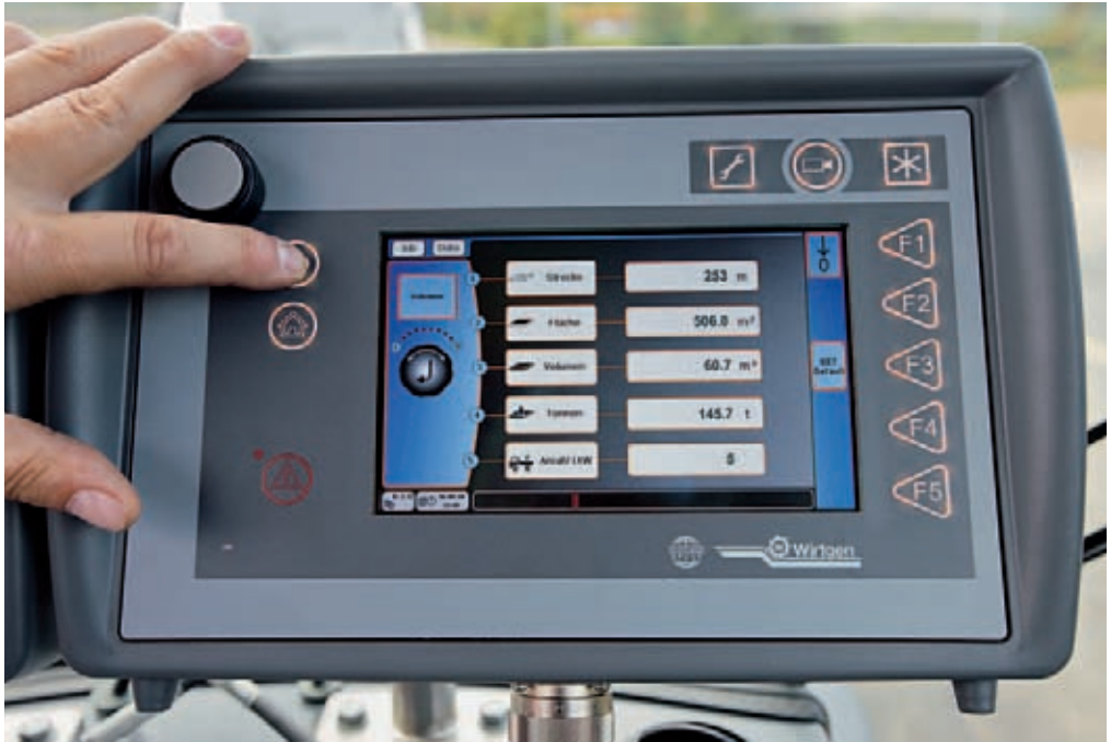
Operating display for job data collection on modern large milling machines
