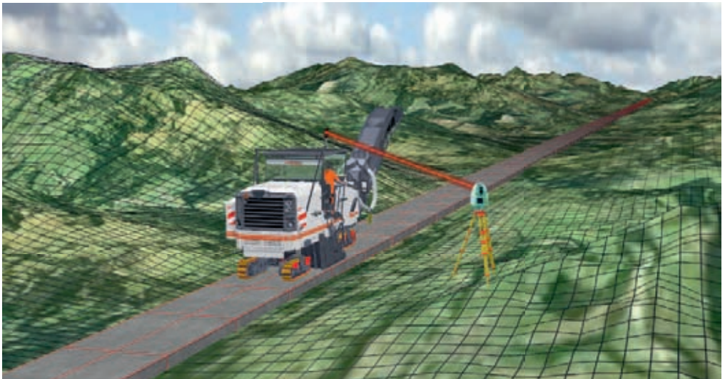
Absolute geodata reference for exact-position determination of milling depth
